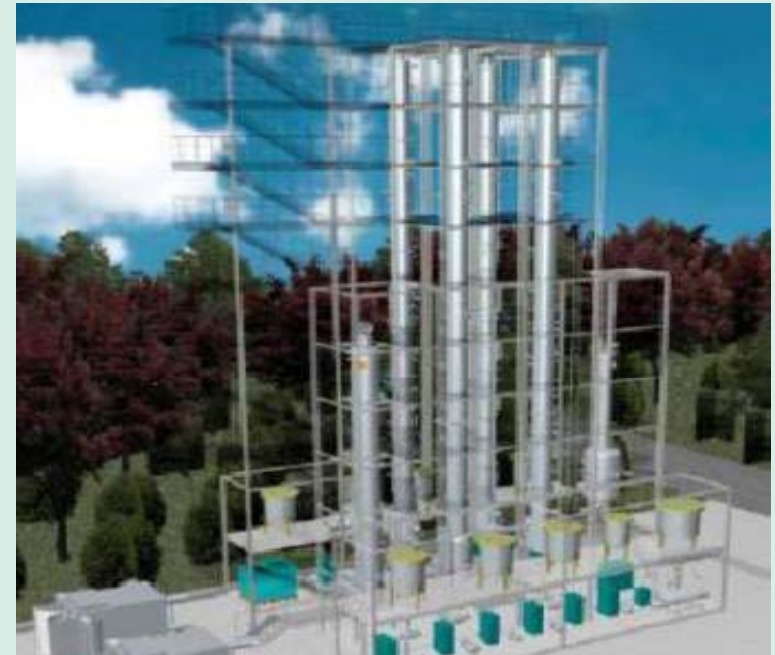
Mobile chemical-absorption system (German Power station)
